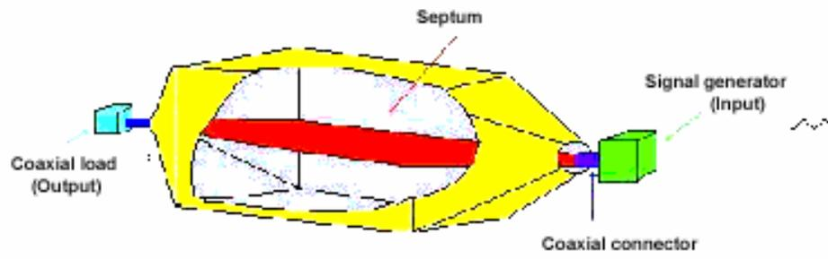
Fig. 1: Diagram of the TEM cell
